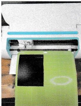
3. Insert the mat into the Cricut, just up to the roller bar. Do Not try to force it any farther in. There are small plastic tabs on either side of the roller bar that will help secure it until you actually load it.
