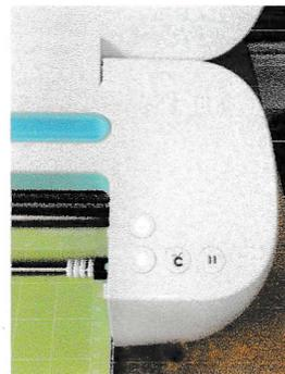
4. Right below the power button is another button with arrows going up and down. This is the Loading/Unloading button. Push that button **ONCE** and the mat will load.
